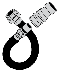
Gas Quick Disconnect
