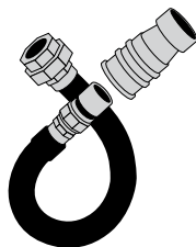
Gas Quick Disconnect
