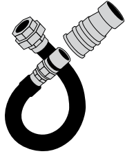
Gas Quick Disconnect
