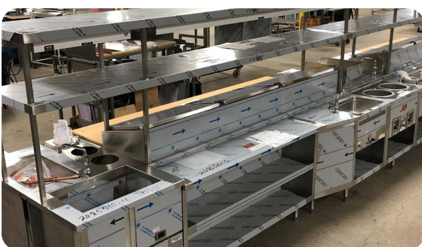
Modified rail unit self-contained that allows you to roll a production refrigerator, freezer or even a heat box under the counter top.
